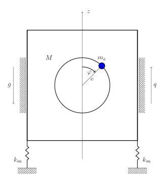
Analysis of the scheme allows to claim its number of degrees of freedom which is 1
